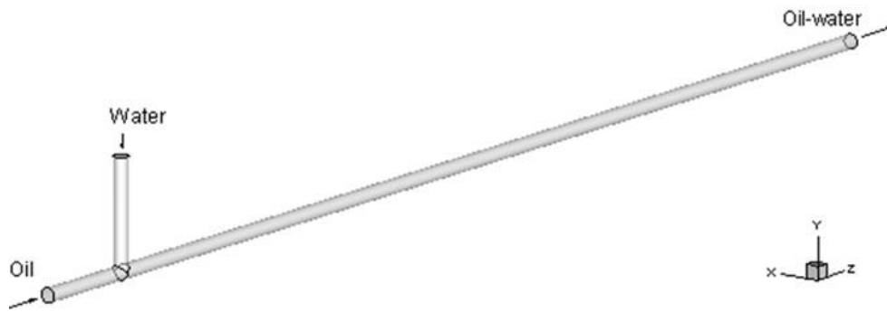
Fig. 2: Pipe geometry for the oil-water flow simulation
