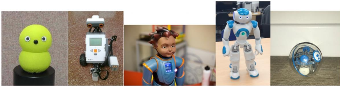
Figure 2. Some commercially available robots. From left to right: Keepon 5 , LEGO Mindstorms NXT 6 , R25 Milo 7 , NAO robot, and Sphero
