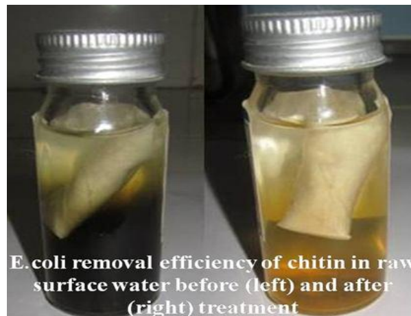
Fig. 6. E. coli removal efficiency of chitin in raw surface water before (left) and after (right) treatment.
