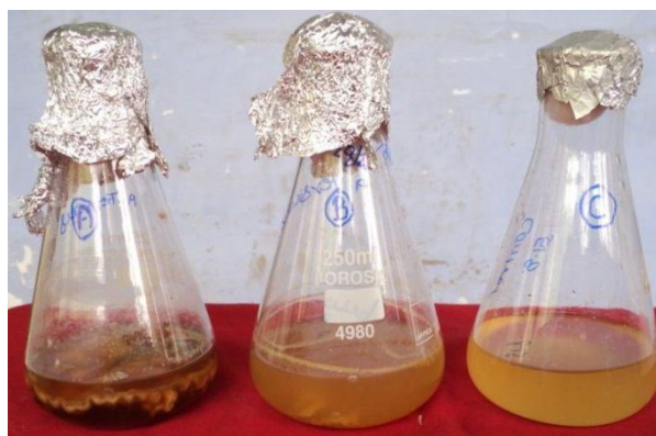
Fig. 2. Figure showing the degradation of polyethylene (high density) by Aspergillus terreus and Aspergillus versicolor .
