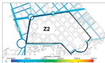
Figure 9. Relative differences of NO x concentration in the District of Plaza de la Cruz estimated for the cases in which the zone indicated in the map above have been applied to different traffic restrictions: traffic reduction 100% (above) and reduction of traffic by 80% (below); and with different redistribution of traffic: with 60% of the traffic diverted to the surrounding avenues (left) and without diverted traffic (right)
