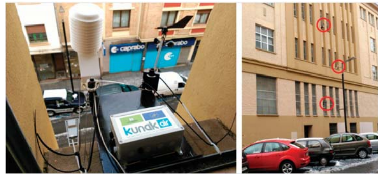
Figure 6. Measurement of atmospheric pollutant concentration and meteorological parameters at different heights in a street canyon in Pamplona as part of the activities of the LIFE+RESPIRA project.
