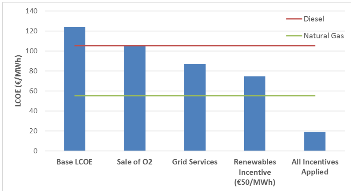
Figure 5. Effect of incentives and supplementary income on effective 2020 base system LCOE with market prices of diesel and household natural gas ex. VAT for reference
