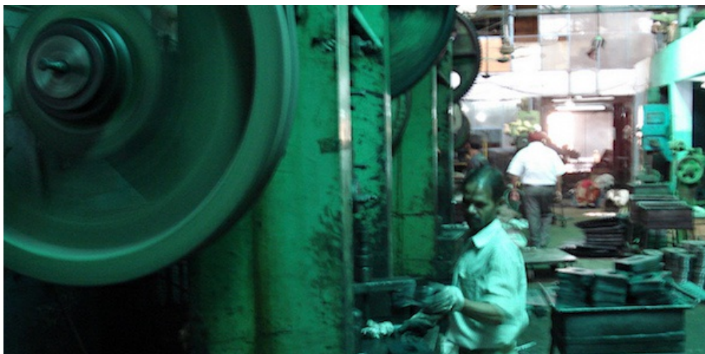
Mechanical punch presses in operation in a factory. Photo credit: ILO in Asia and Pacific , Flickr , CC BY-ND 2.0 .
