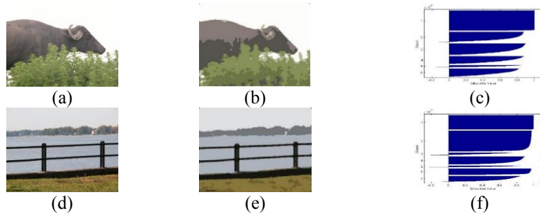
Fig. 8. Cluster performance measurement using silhouette visualization. (a) buffalo: color image (b) buffalo: final segmentation (c) buffalo: silhouette visualization (d) sea: color image (e) sea: final segmentation (f) sea: silhouette visualization
