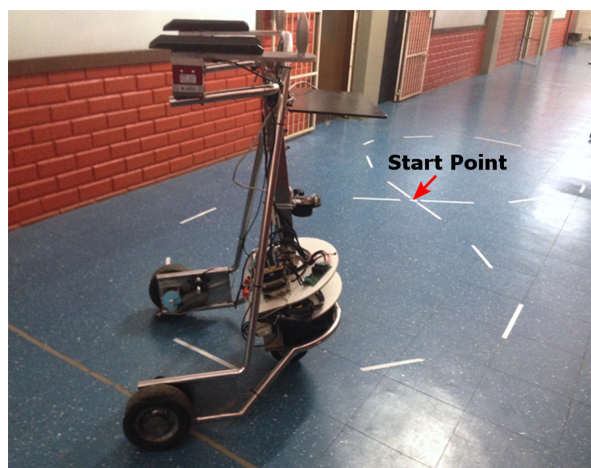
Figure 3.4: Experiment 2, where the users were asked to follow a lemniscate curve indicated on the floor.
