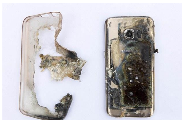
Figure 1.2 – Samsung Galaxy Note 7 damaged by battery explosion (Daily Mail Journal, 2016)
