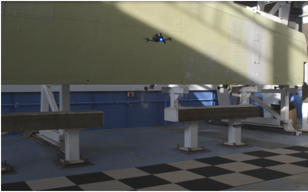
(a) The concept of using the onboard UV-light for flow penetrant testing.
