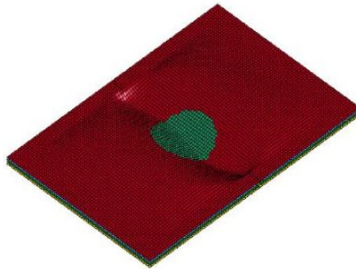
Figure 5 CAI failure mode of the numerical model
