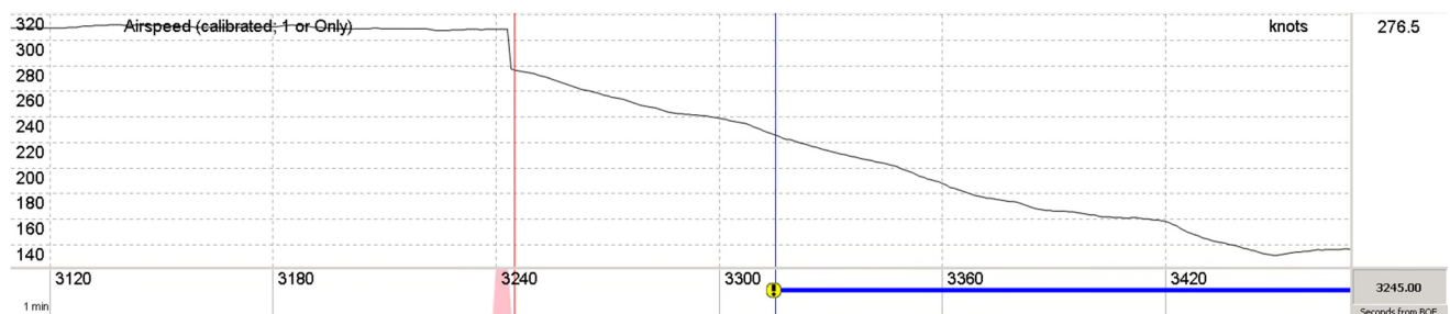
Figure 4: Synchronization error: The red shaded area at the bottom indicates that software detected a synchronization problem, which caused a sudden sharp jump in the recorded airspeed. Source: Author, taken from ADI EMS software.
