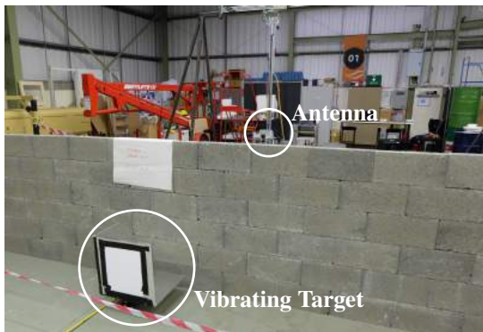
Figure 6: Experimental set-up used for through-wall measurements.
