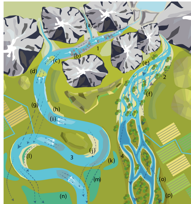
Figure 1. Illustration of catchment complexity: scales and features that influence hyporheic exchange flows. Spatial changes in surface topography, land use and vegetation drive geomorphological and hydrological changes at valley and reach scale. At catchment scale, variations in surface topography shape valleys and channel types. Feature 1 refers to confined valleys characterized by straight channels, meandered and braided, and the following floodplain features: scour holes and gravel splays (a). The straight channel presents in-channel cascades (b) and geomorphic features. Feature 2 refers to braided channel morphology with multi-thread channels, an undulating floodplain of bars and islands. In-channel geomorphic units are several types of bars (e), such as mid and lateral bars, and vegetated islands (f). Feature 3 represents a sinuous-meandering floodplain with occasional oxbow lakes and backwater swamps (m, n, k) and in the channel: longitudinal bar (c), transverse bar (d), counterpoint bar (h), pond-riffle (i), point bar (l), chute channel (j). Feature 4 indicates an anabranching valley with multi-thread channels including abandoned channels (o) and backwater swamps (p). The channel can be quite deep and includes islands covered with vegetation.
