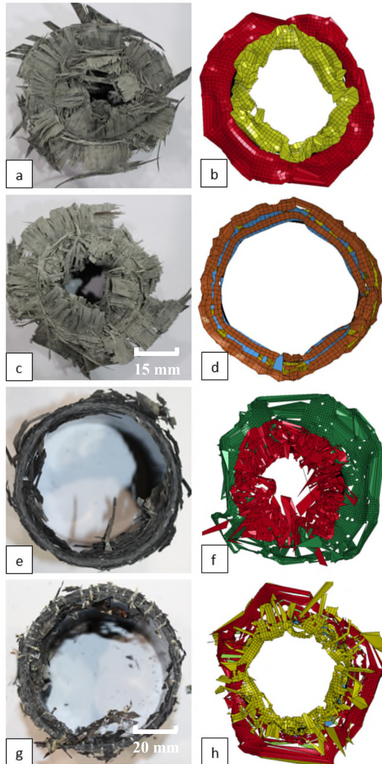
Fig 13. Plane view of the tested GFRP and CFRP under impact load a) non-stitched GFRP experiment b) non-stitched GFRP FEA c) stitched GFRP experiment d) stitched GFRP FEA e) non-stitched CFRP experiment f) non-stitched CFRP FEA g) stitched CFRP experiment h) stitched CFRP FEA.
