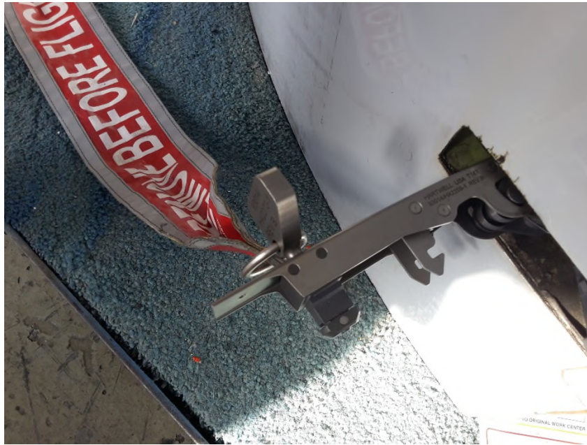
Figure. 4 Modified A320 family engine FCD with new latch and key - ‘remove before flight’ flag assembly.
