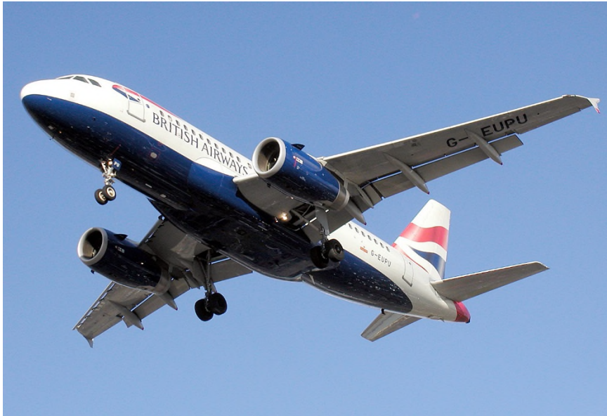
Figure. 1 A British Airways Airbus A319-100, where the (blue-painted) fan cowl doors (FCDs) surrounding the engines are shown (photograph by Adrian Pingstone).
