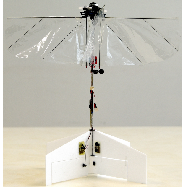
Figure 1: The FlowerFly with onboard camera and control system for pitch-, yaw-, and roll-control controlled by three servos.
