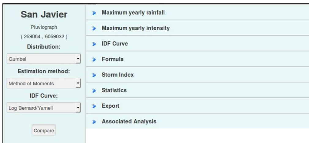
Figure 7. Visualization and analysis of rainfall intensity for a pluviographic gauge (San Javier) included in WEBSE IDF .
