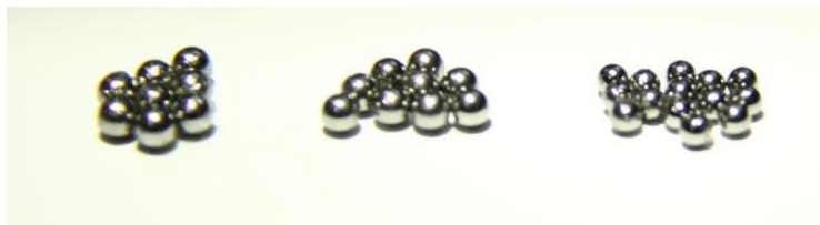
Fig. 7: Balls for simulation of backlash
