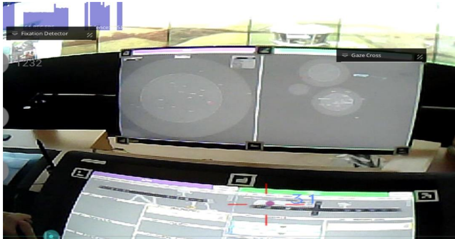
Figure 7. ATCO shifting attention from Shannon to Cork airport to pay attention on the runway activities on the EFS (fixation shown as red-cross recorded by eye tracker)
