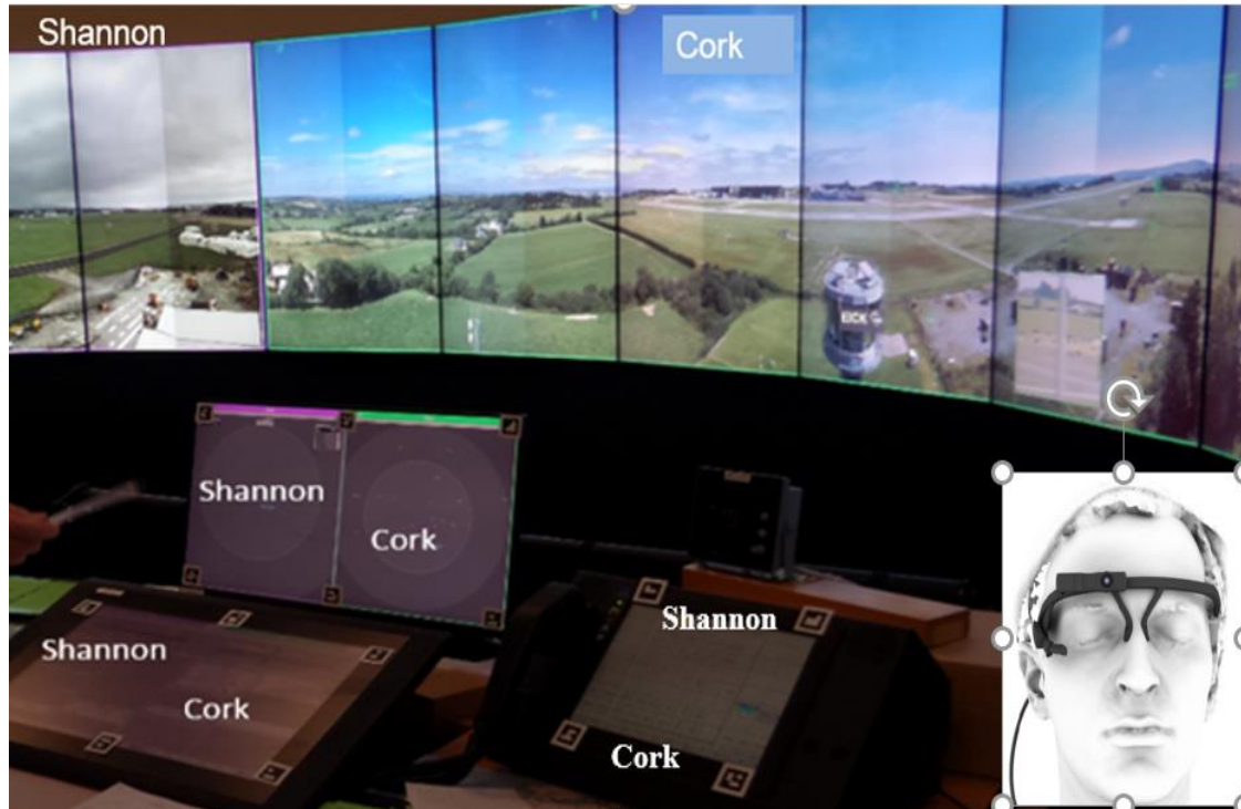
Figure 2. ATCO's using Pupil Pro Eye Tracker interacted with RTM comprised OTW, RDP, EFS and VCS (left-hand side are Shannon airport, right-hand side are Cork airport) for Multiple Remote Tower Operations.
