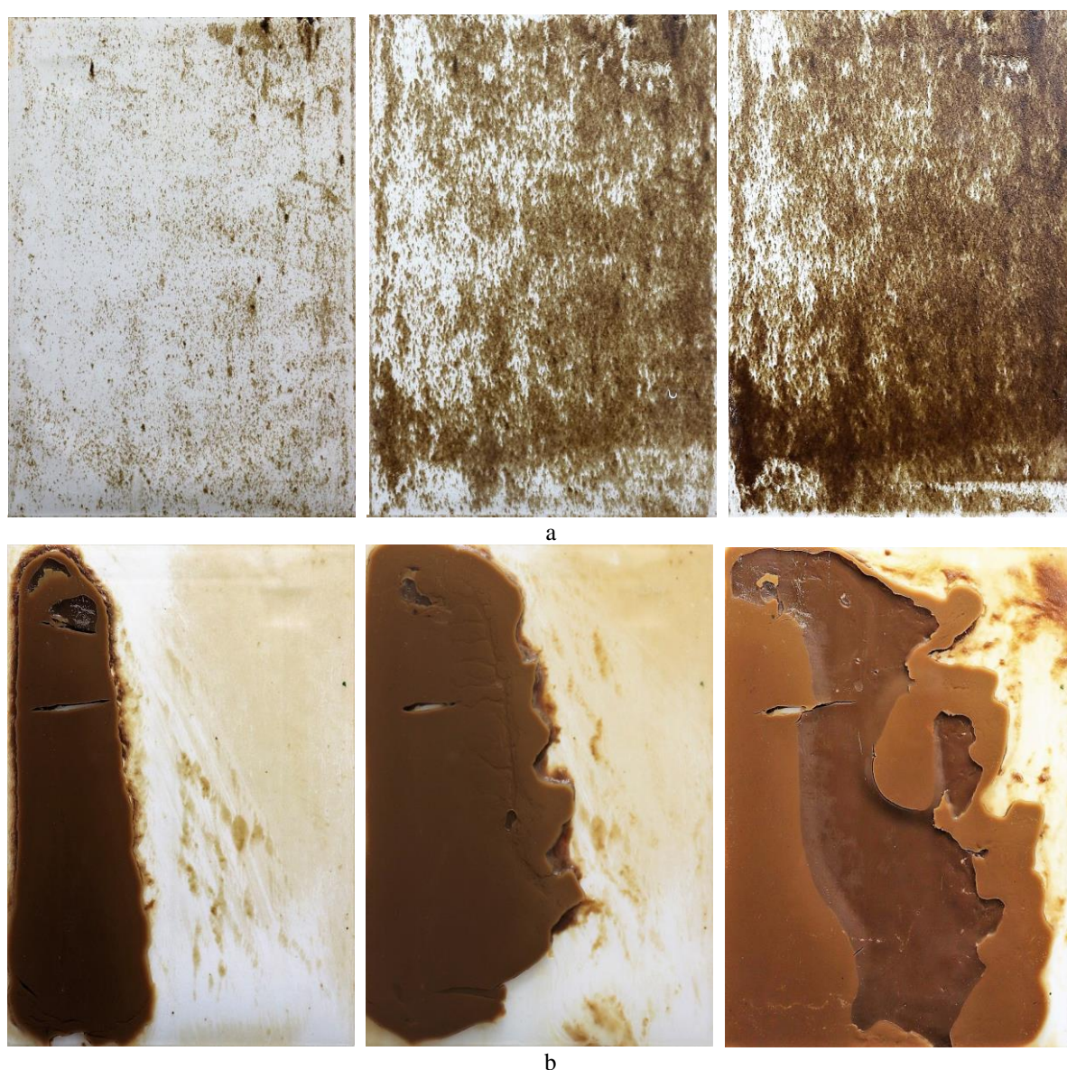
Figure 5: Examples of progressive sludging in 1-4 hour timeframe: (a) municipal, and (b) industrial MBR sludge sample, MLSS = 8-12 g.L -1 , U_a = 0 m.s -1 .
