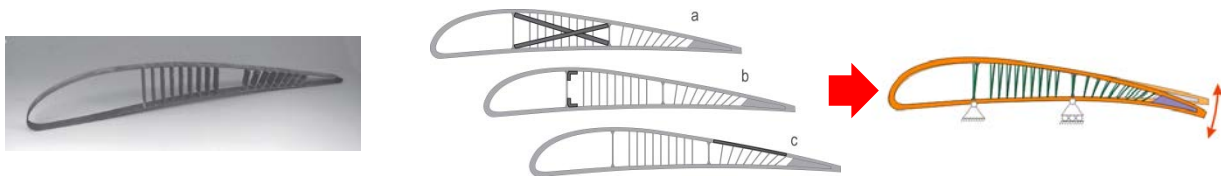
Figure 3: Belt-Rib concept showing demonstrator (left), activation (centre) and deformation (right) [31]
