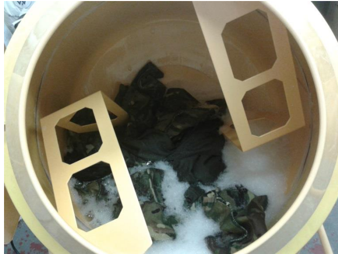
Figure 4-4 Example of laundering with the cement mixer
