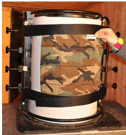
Figure 3-2 Typical specimen mounted for ballistic testing
