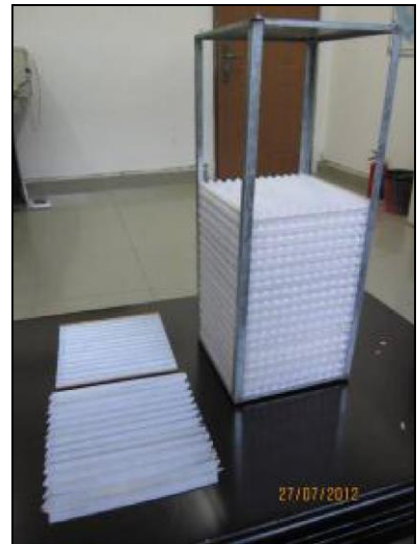
Figure 4-27: Zhang's and Li's actual assembled total heat exchanger [181].
