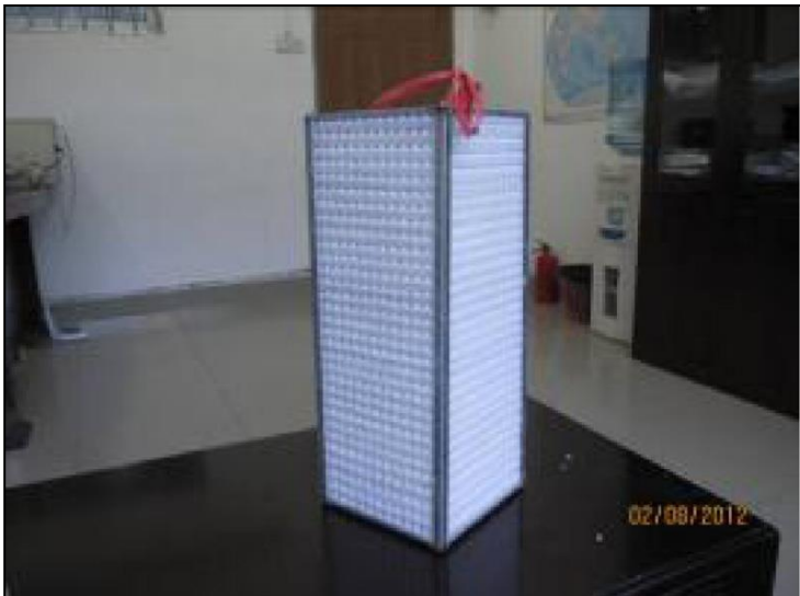
Figure 4-27: Zhang's and Li's actual assembled total heat exchanger [181].
