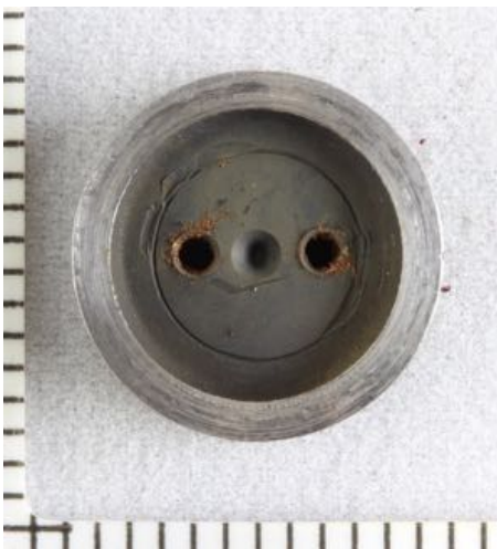
Figure 5.10 Inside of cartridge case showing bolster marks and flash holes.
