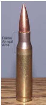
Figure 2.11 A round of ammunition showing discolouration of the cartridge cases where flame annealing has occurred (the neck and shoulder area) [12].
