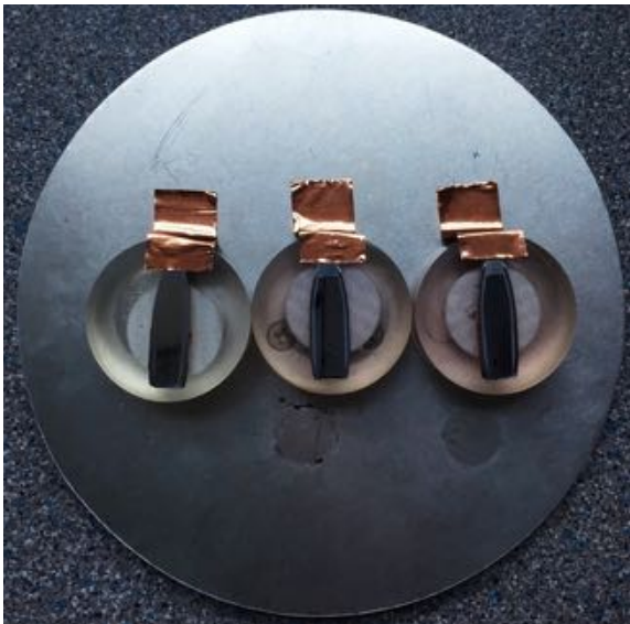
Figure 5.15 Sectioned projectiles secured to 127mm mount with conductive copper tape to prevent charging.
