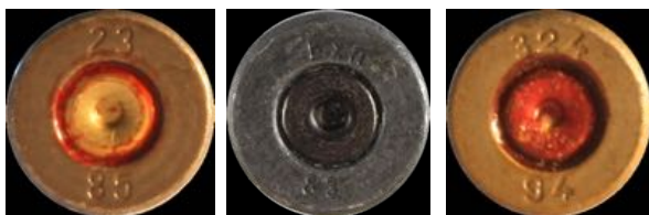
Figure 6.25 Photographs of primer annuli and lacquer from (left to right) Hungary (23/85), Czech (bxn/83) and Romania (324/94), showing variation (and absence) in lacquer.
