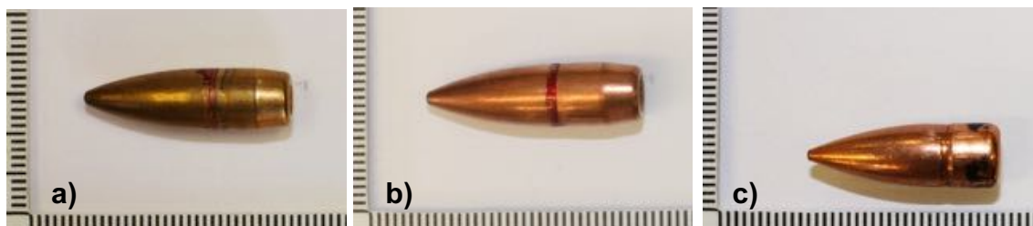
Figure 6.1 Photographs of projectiles from a) Albania (11/89/3), b) Russia (539/76) and c) South Africa (13/88), showing variation in jacket colour, lacquer, and shape.
