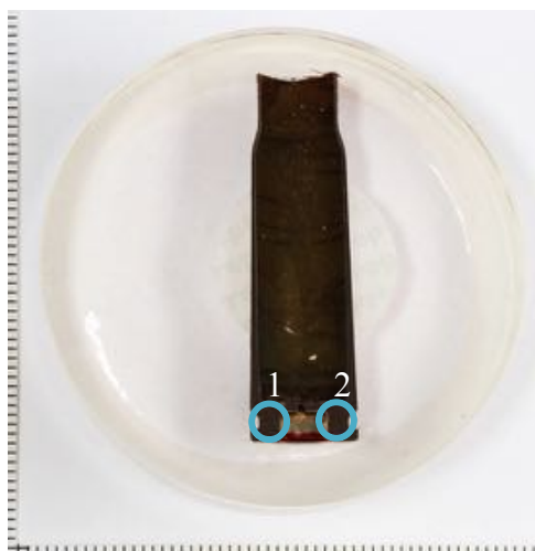
Figure 5.13 Sectioned cartridge case showing two points for XRF analysis.
