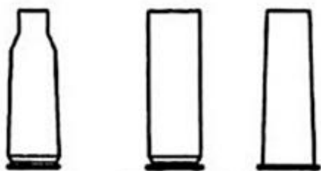
Figure 2.8 Cartridge case types (from left to right): bottlenecked, straight, tapered [38].
