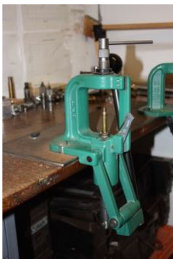
Figure 5.1 RCBS Loading press set up with pulled cartridge case seated.
