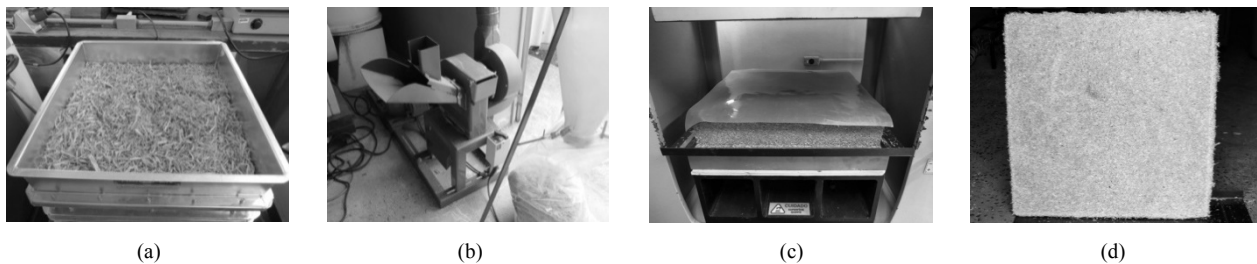
Figure 1: (a) Sieve shaker, (b) knife mill, (c) mattress particles in the hydraulic press with heating, and (d) high-density homogeneous particleboards of SCB and the polyurethane resin based on castor oil.
