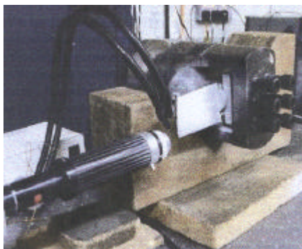
Figure 4. The electronic speckle interferometry system.
