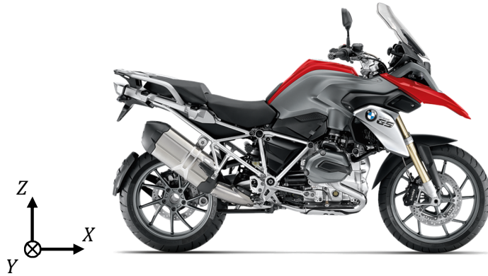
Figure 2 – Test motorcycle with the global reference coordinate system ©BMW AG.
