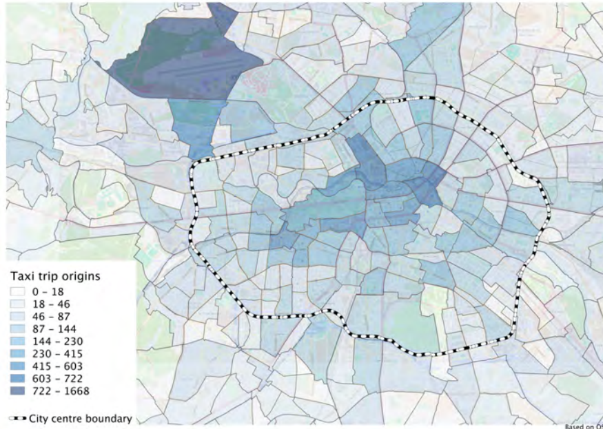
Figure 3: Daily taxi demand in Berlin by zone of trip origin. High demand, marked in dark blue, originates mainly in most central parts of the city center and at Tegel Airport.
