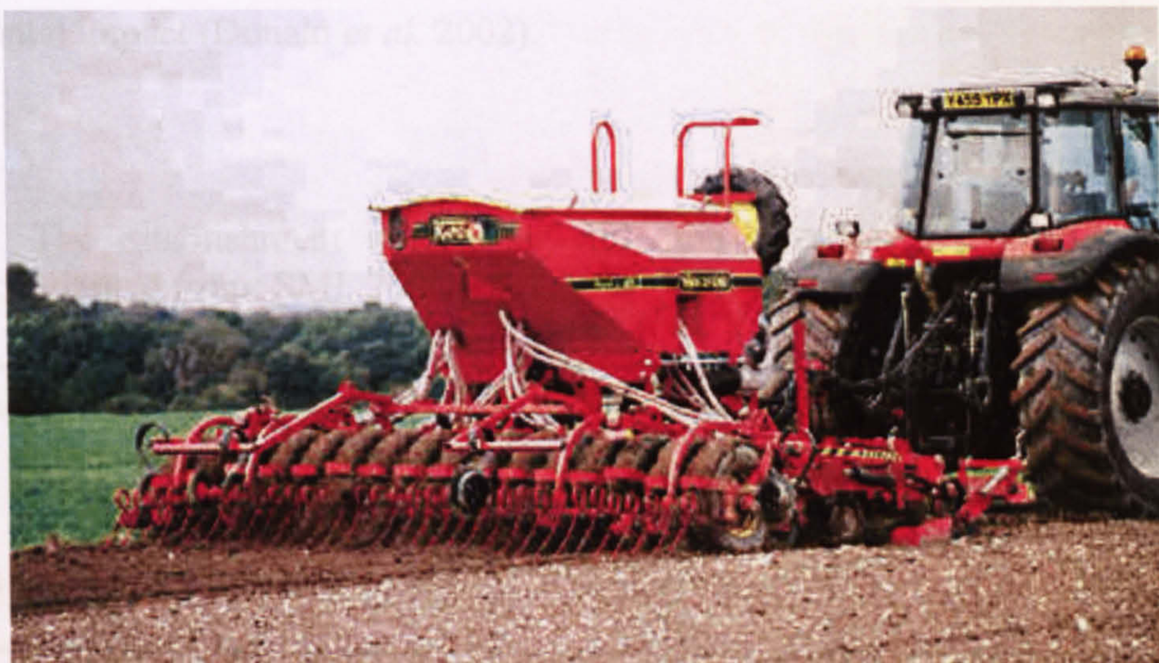
Figure 1.3. Non-inversion tillage equipment: Vaderstad combination drill (Source:
