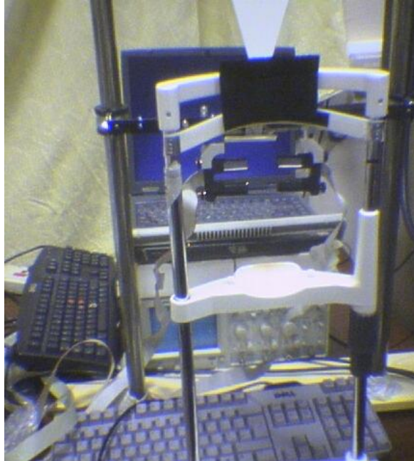
Figure 1.1. Overall experimental set up. The head and chin rest is visible in the foreground; beyond that are the eyetracking LEDs for left and right eyes, and at the rear, a laptop PC. A keyboard is positioned just beyond the head and chin rest to record subjects' manual responses. The eyetracker is displayed in the configuration used in the patient study (Chapter 6). To improve comfort and make the paradigm as tolerable as possible, the eyetracker LEDs were removed from their plastic helmet-frame and mounted on the head and chin rest. The patient's head was then supported at the back with a Velcro-fastened strap. In the other studies the LEDs were kept mounted on the helmet-frame (Photograph: A. Nuruki).
