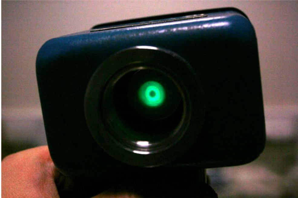
Figure 4-3. An electroviewer is used to visualize the near-infrared radiation from the Diomed laser.
