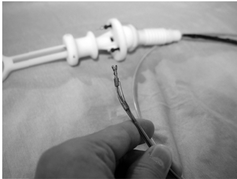
Figure 2-7. A 3.2mm diameter articulating grasper with an “intuitive” control interface. (Personal photograph.)
