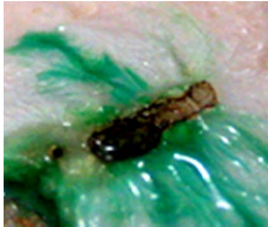
Figure 3-3. A linear incision by made an 805 nm Diomed laser in chicken tissue stained with ICG. Features of the ablation crater are typical of ICG-mediated ablation.
