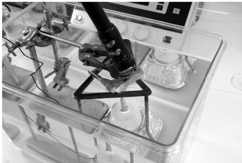
Figure 3-41. Acoustic "fingerprinting" experimental setup with CO 2 laser, tissue, and needle hydrophone submersed in a water bath.
