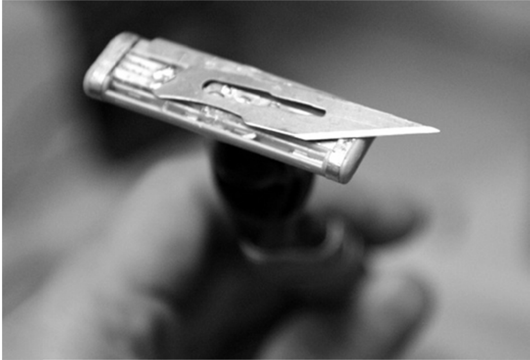
Figure 3-45. A crude attempt at a vibrating blade using a commercial vibrating shaving razor handle.
