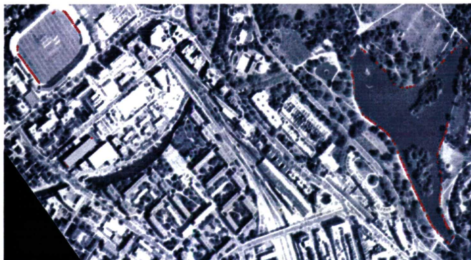
Figure 4.12: Plot of 376 planimetric match points on the registered London Regent's Park image.
