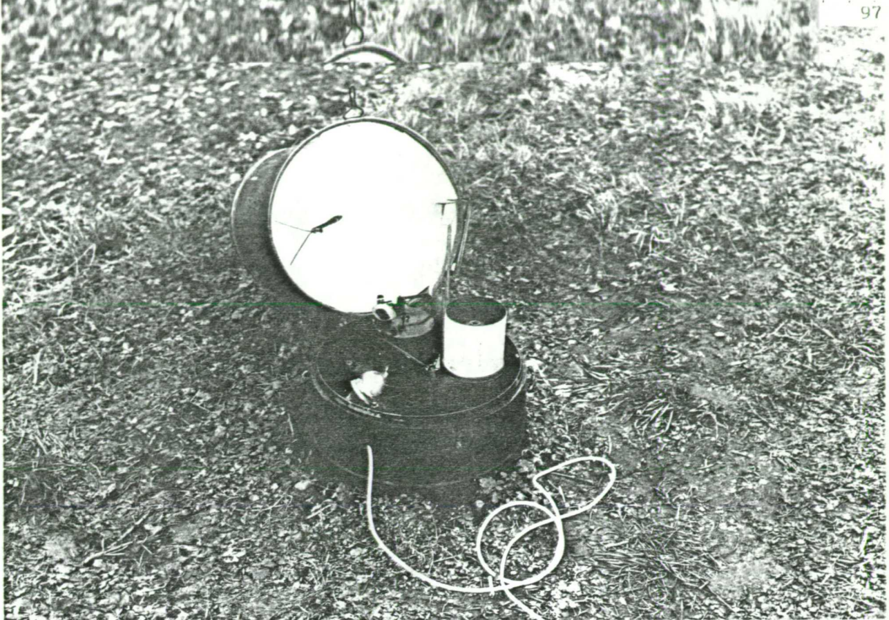
Fig. 4.5 Opened tilting-siphon rain gauge showing 40 watt light bulb and polystyrene insulation to prevent frost damage.
