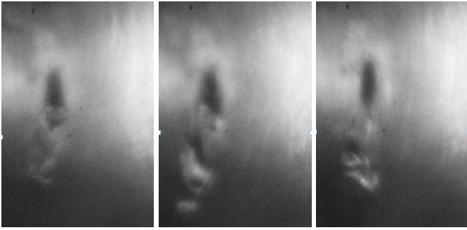
Figure 19. Image sequence showing fuel discharge after needle closure
