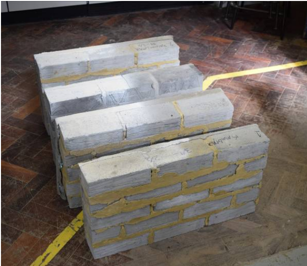
Figure 2. Strengthened specimens with UHPFRC layers with various thicknesses
