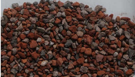
Fig.1. Recycled aggregates used in the research of RAC-RCBA
