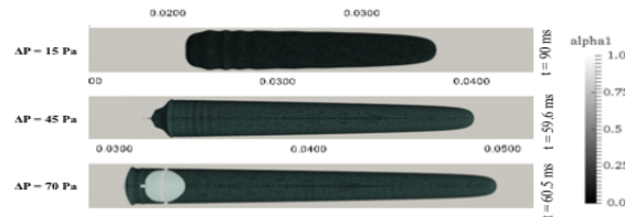
Fig. 6. The effect of the APD on the resulting elongated vapour slug break-up regime (FC-72, \delta_{\text{film}} = 50 \mu\text{m} , D_{\text{channel}} = 3 mm, \sigma = 0.084 N/m, q'' = 0 W/m 2 ).
