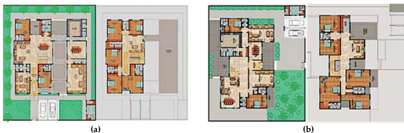
Figure 11. Two Typical House Models in Shaubat Al Wuttah Urban Community: (a) Ground Floor and (b) First Floor Plans. The Expandable Area is Shown in Dark Gray on the First Floor. (Source: Al Ain Municipality).
