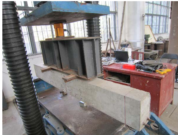
Figure 3. Flexural testing setup
