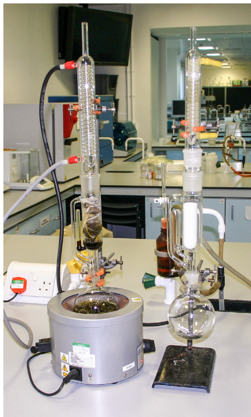
Figure 5 Soxhlet extraction apparatus: (left) extraction of caffeine from teabags; (right) the use of a porous thimble within the Soxhlet apparatus to extract caffeine from loose tea
