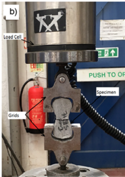
Fig. 3. a) Set up of direct tensile strength test using a) dog-bone shaped specimens for hybrid fibre composites direct tensile tests, and b) Standard Briquette used for nano-fibre composites direct tensile tests (all dimensions in mm)
