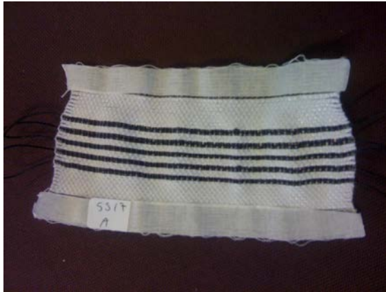
Figure 20: 4/4 Hopsack Structure: TPU/CNT Continuous Weft with elastic
