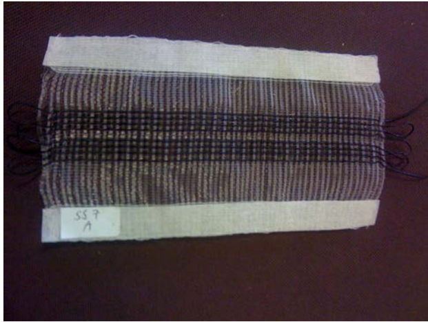
Figure 17: Float Structure: TPU/CNT Continuous Weft with nylon
