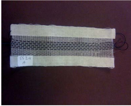
Figure 21: 8/8 Hopsack Structure: TPU/CNT Continuous Weft with nylon
