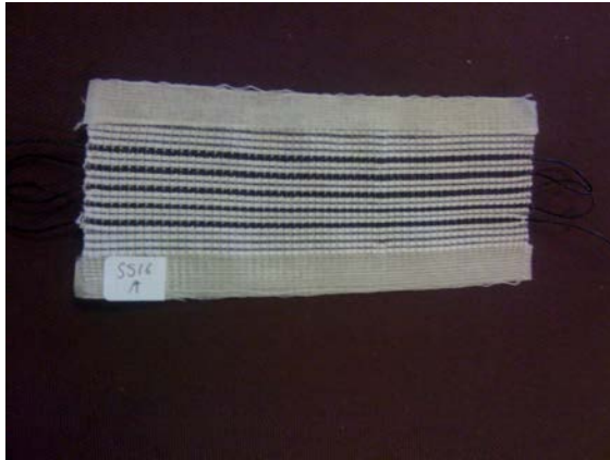
Figure 19: 4/4 Hopsack Structure: TPU/CNT Continuous Weft with elastic and nylon
