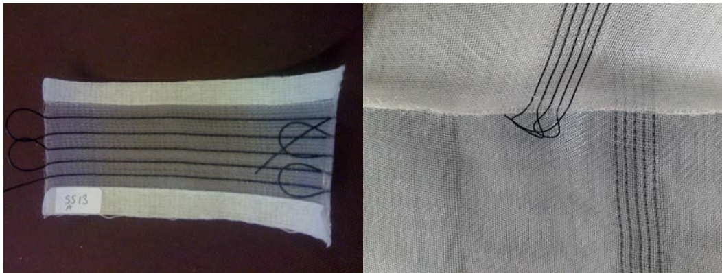
Figure 18: Sateen Structure TPU/CNT Continuous Weft with nylon
