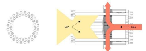
Fig 1. Left: 48 pipes oriented in two concentric circles. Right: Solar irradiation hits the pipes on the inside of the circles. Combustion gases flow radially through a fin package connected to the pipes.
