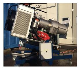
Fig 2. The hybrid receiver mounted on a SunBox engine and inclined 15°
