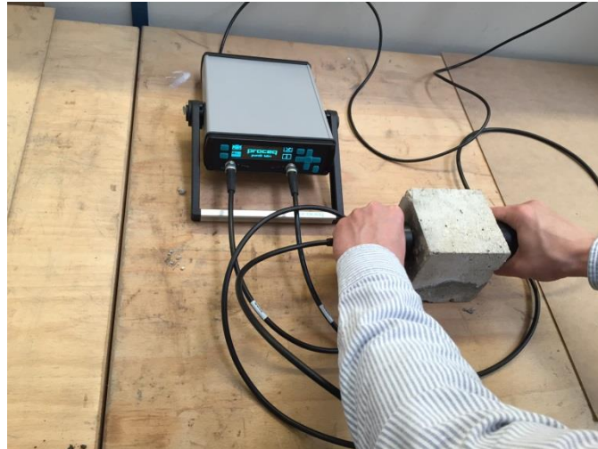
Figure 7. UPV tests on cubes
