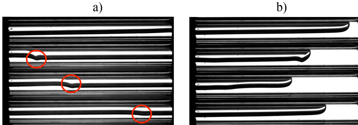
Figure 10. a) Stratified flow with highlighted ripples; b) Oscillating bubble.
