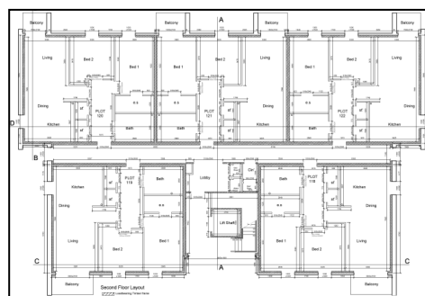
Figure 5 Building second floor plant
