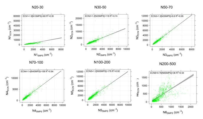
Figure 1 - Comparison between ECN UFPM and ECN SMPS size classes (one month data). N1 to N6 represent the individual particle size classes of the size-resolved instruments.
