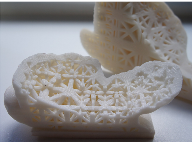
Fig. 9 The Stanford bunny printed in ABS using the primal open cell structure.
